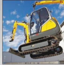
**2 lifting lugs** to easily move the entire machine
