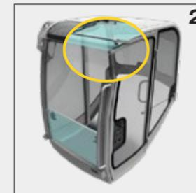
The upper windshield can be pushed under the cabin roof. The lower pane serves as splash protection.
