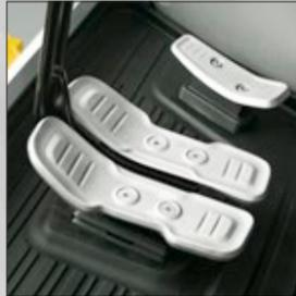
**Sensitive operation** and exact work using hydraulic pilot controlled pedals
