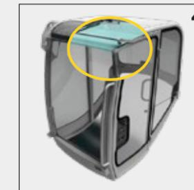
If necessary, both windows are pushed below the cabin roof where they are stored safely.
