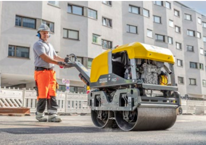
Long center pole makes steering and turning easier, particular on small surfaces.
