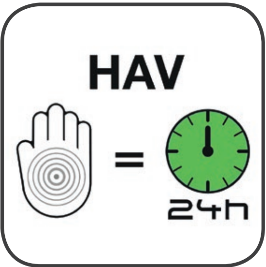
Low hand-arm vibration values (< 5 m/s²) for work comfort, even when using the WP1550 for longer periods.
