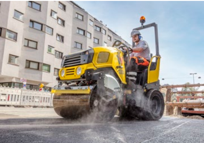
Waisted design: for an unobstructed view of the drum edges, the machine surroundings and the construction site.
