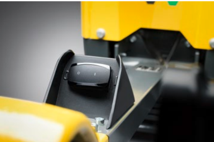
The switch has been made easily accessible on the center pole for the operator.
