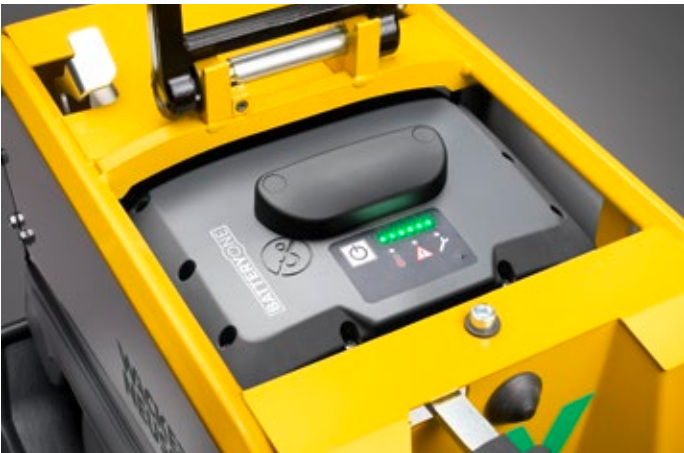
With one battery charge, the APU3050e compact up to 333 m² soil*.
