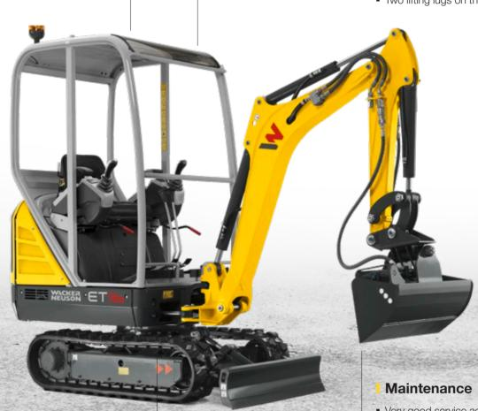
Very good service access due to the large rear engine hood and removable floor plate in the cabin
